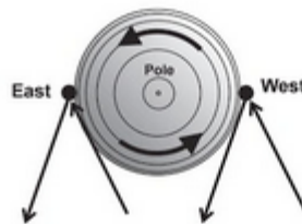
Figure 12.2 The Doppler effect acting twice for reflected light from planets
